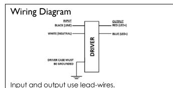
Lead-wires are 18AWG 105C/600V solid copper
